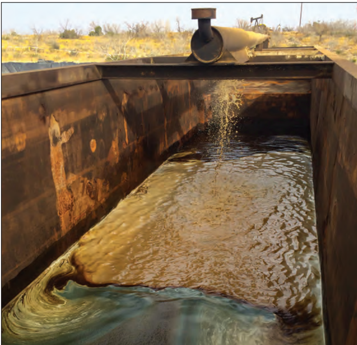
Fracking wastewater is laden with the many chemicals used in fracking fluid, as well as radioactive material, heavy metals and other compounds found in the targeted rock.
